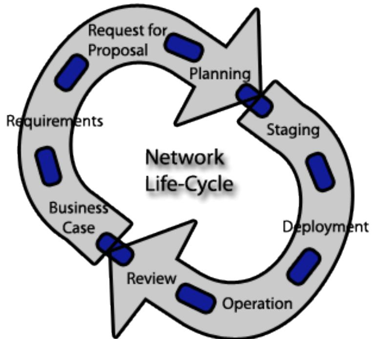
*Network Life Cycle (NLC) - describes the stages of network design, staging, deployment and operation.*
